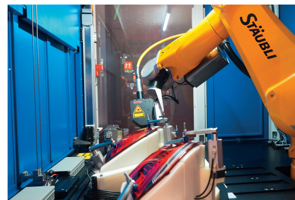
Fig. 3. View of the laser welding workstation from Leister – equipped with a 6-axis robot at K show. © Hanser/Schröder
